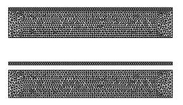
The global moving mesh is compatible with the interface: a triangle of the global mesh belongs either to the fluid region or to the structure region.
