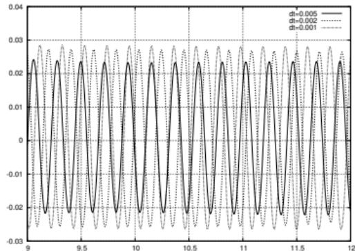
For  $\Delta t = 0.005$ , the amplitude is 0.022 m, the frequency 4.72 Hz,
